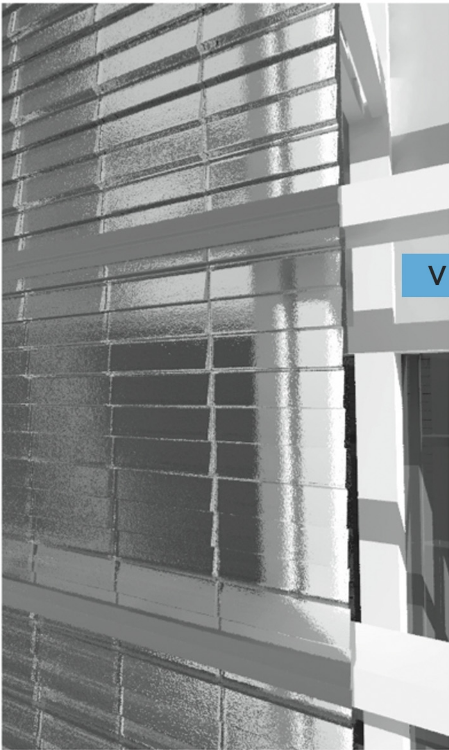
Figure 28. Building 3D model showing a portion of the façade with the cast glass virtual model
