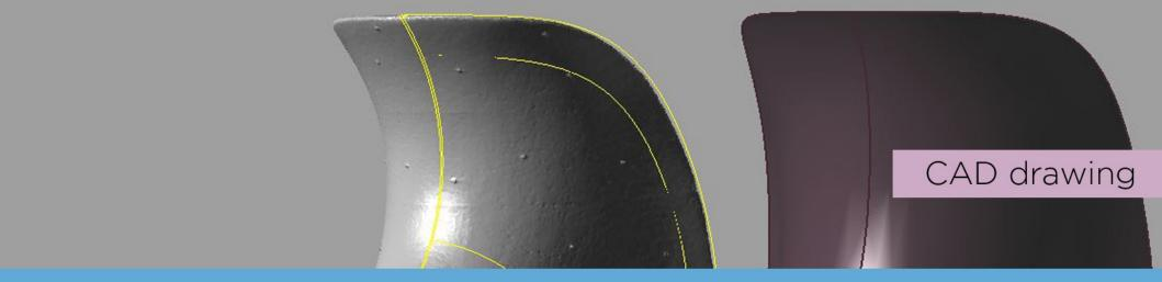
The finished 3D scan data on the left, was used to create an idealised CAD model. We cut cross sections through the model and used these to create a symmetrical design with set measurements on specific lengths and diameters. This CAD drawing was then handed to the structural engineers.
